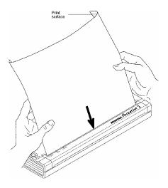
FIGURE 9. Inserting a sheet of paper
